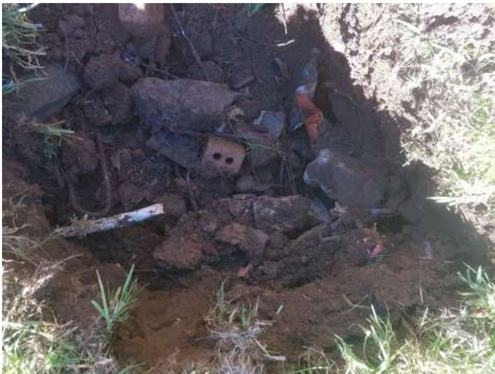
Photo 6: Test Pit 61 with rubble fill including bricks, concrete, plastic and steel reinforcement pieces.
